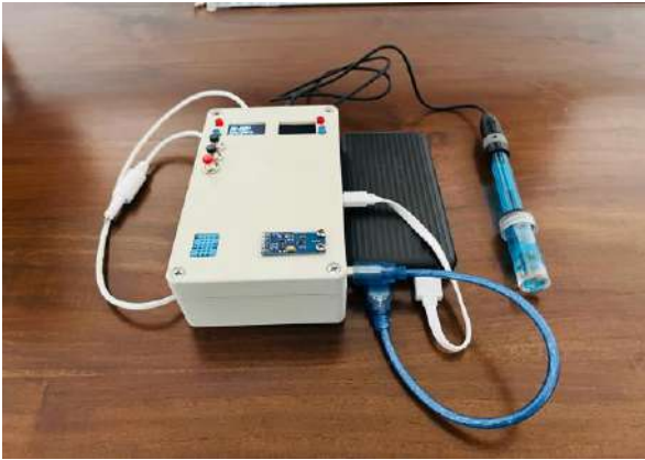
Figure 4: Final Functional Prototype of the HypoSense
