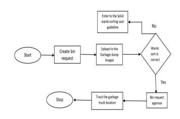
Figure 8. Process flow diagram for citizens bin request process
