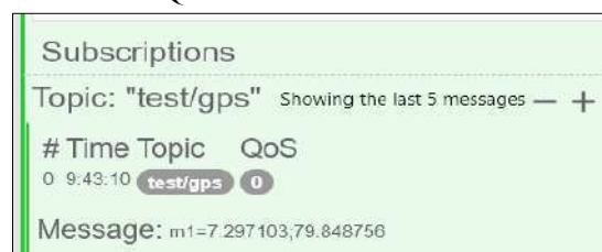
Figure 5. Test the publication of data through MQTT Lens
