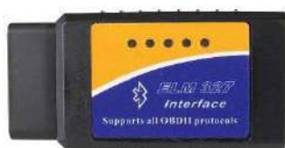
Figure 2. ELM 327 Bluetooth Scanner
