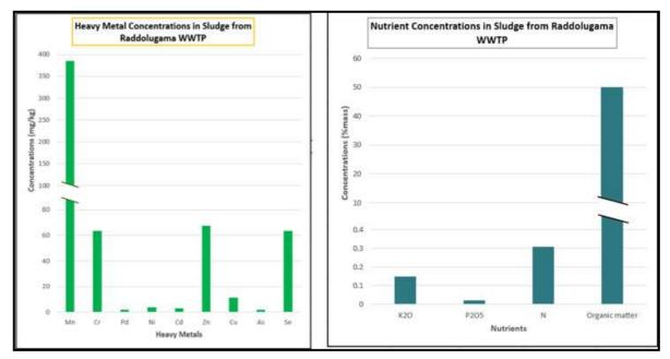
Figure 8. Heavy metal concentrations in sludge from Raddolugama Sewerage Treatment Plant dated 22/06/2021 and Nutrient concentrations of sludge from Raddolugama Sewerage Treatment Plant dated 22/06/2021
