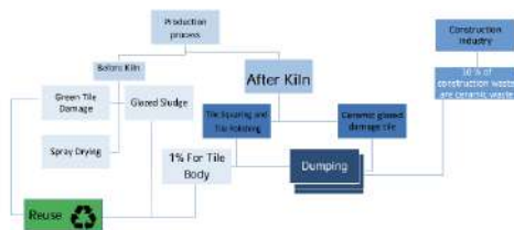
Figure 2. Production and waste generation process of ceramic tiles.
