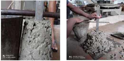
Figure 6. Conducting Slump test in the lab
