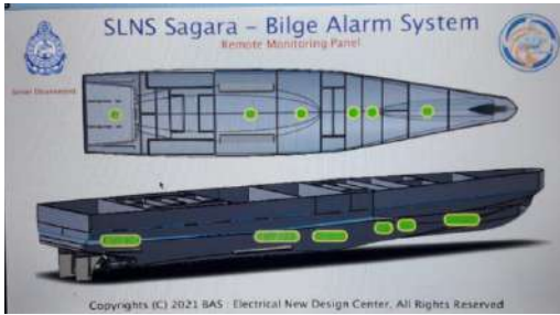
Figure 2. Bilge Alarm GUI
