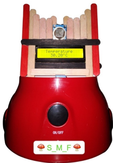
Figure 3: IOT Environment Factors monitoring Device
