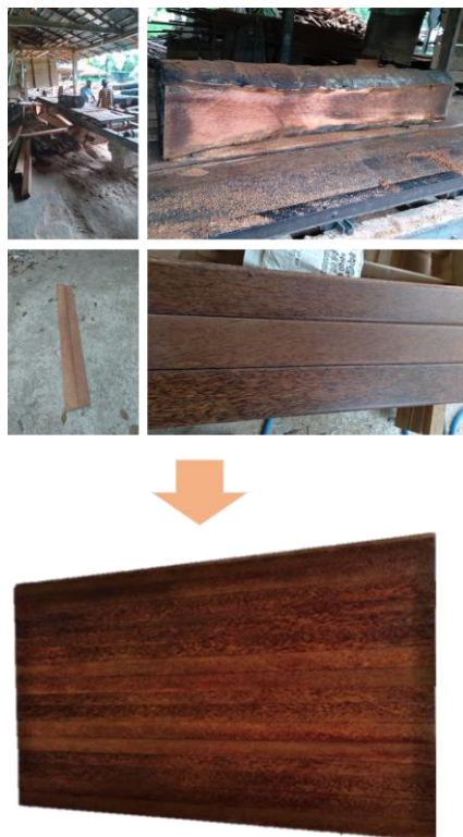
Figure 9: Processing of Cocowood tile
