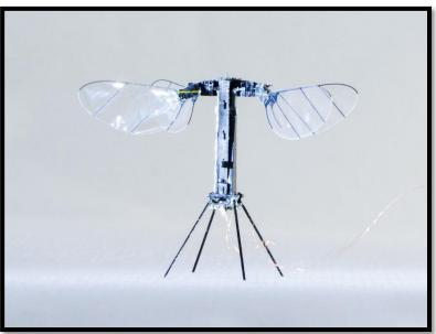
1. RoboBee—a flying machine half the size of a paperclip that could flap its pair of wings 120 times a second. It was always tethered to a power source, limiting its freedom. Now, though, RoboBee becomes RoboBee X-Wing and consists of solar cells and an extra pair of wings that carries the weight of this very small drone.
