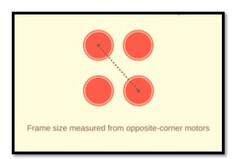
60. The frame size of a quadcopter is the distance from opposite corner motors. So if you measure from the front left motor to the back right motor, that distance (in millimeters) is the frame size.
