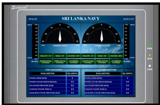
Figure 5. Designed HMI for Closed Bridge
