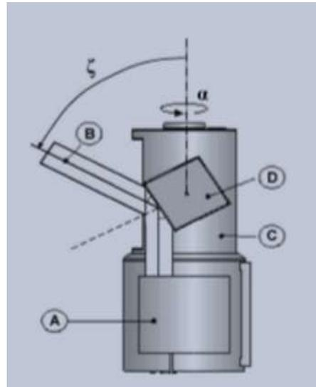
A TLS needs a two axis that are capable of freely rotating in two different planes like modern TS for surveying a different part of the target in different planes. These two-rotation axis directions can be simply explained as the vertical and horizontal.
