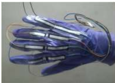
Figure 2: Data glove with flex sensors
