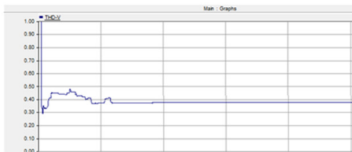
Figure19: Impact to the voltage harmonics at high irradiance
