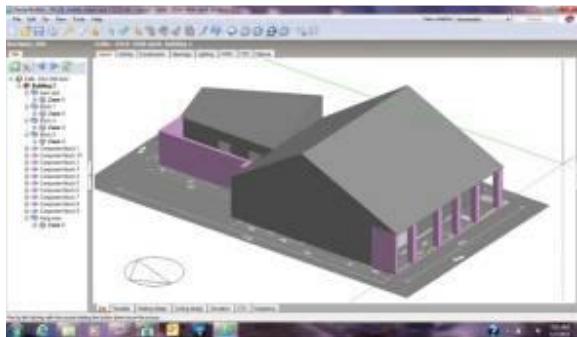
Figure 2: Calibrated model with integration of openings at the roof level and courtyard levels for nocturnal ventilation by stack effect
