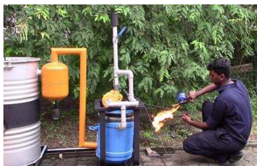
Figure 6 : High flammable syngas
