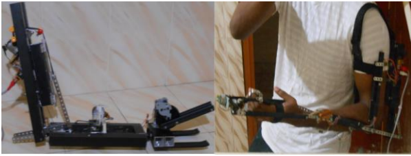
Figure5. The mechanical arm and the frame worn around the paralysed patient's weakened arm
