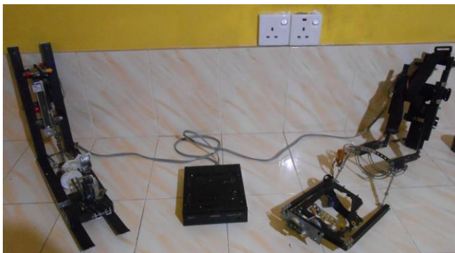
Figure1. The mechanical-arm, Junction box and the frame
